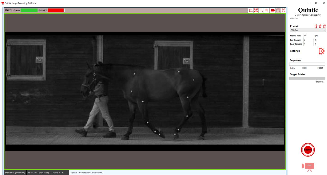
The Quintic Image Recording Platform should then open with a live view of the camera(s) which are plugged into the PC and are configured correctly (Cam IDs). The first time the Quintic Image Recording Platform is opened, it will open with 1 camera, regardless of how many you have plugged into the PC. This can be changed by going into the Settings, then Acquisition. Please read on for further information.
