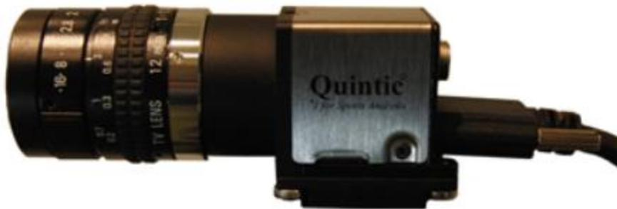
Connect the USB3 Camera with the supplied USB3 cable into a USB3 port on your computer. Please do not plug the USB3 camera into a USB2 port as this can have a detrimental effect on the cameras capabilities.
