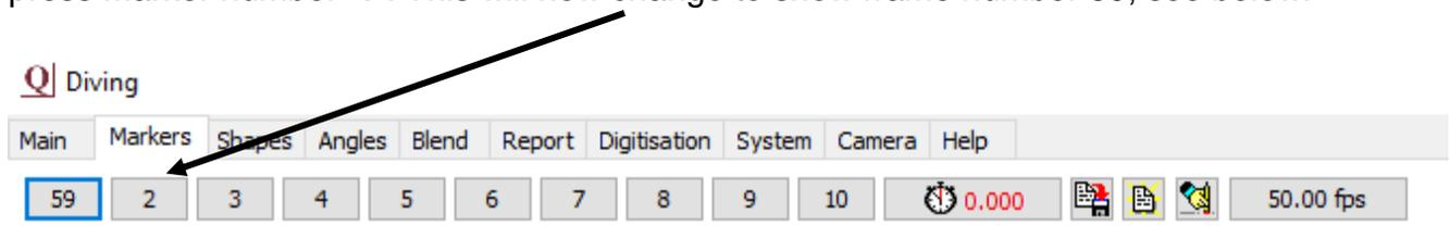
Set the marker's name by right clicking on the frame number and typing in the box to the right, then click the tick box.
