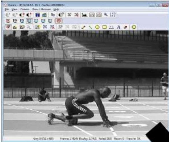
To use the AOI function select ‘Set New AOI’ from the camera tab or click on the ‘Set New AOI’ button on the toolbar.
